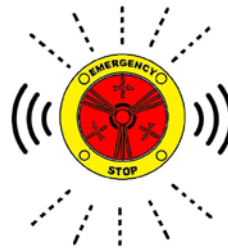
Pulsante + luce lamp.te veloce e sirena / Button + fast flashing light and siren
